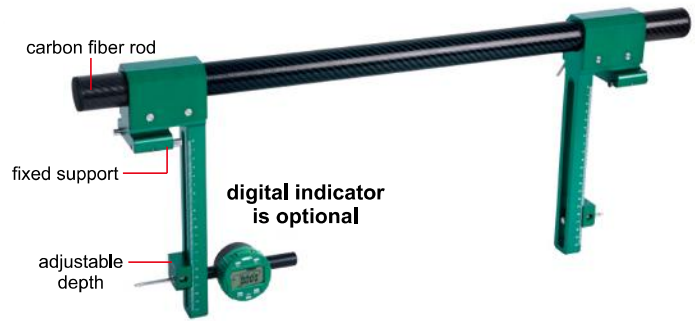
measure inside diameter, minimum diameter is 220mm
